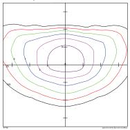
Horizontal Footcandles Scale: 1 Inch = 25 Ft. Light Loss Factor = 1.00 Lumens Per Lamp = N.A. (absolute photometry) Luminaire Lumens = 25151 Mounting Height = 25.00 Ft Maximum Calculated Value = 7.11 Fc
