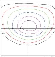
Horizontal Footcandles Scale: 1 Inch = 25 Ft. Light Loss Factor = 1.00 Lumens Per Lamp = N.A. (absolute photometry) Luminaire Lumens = 24635 Mounting Height = 25.00 Ft Maximum Calculated Value = 7.55 Fc Arrangement: Single
